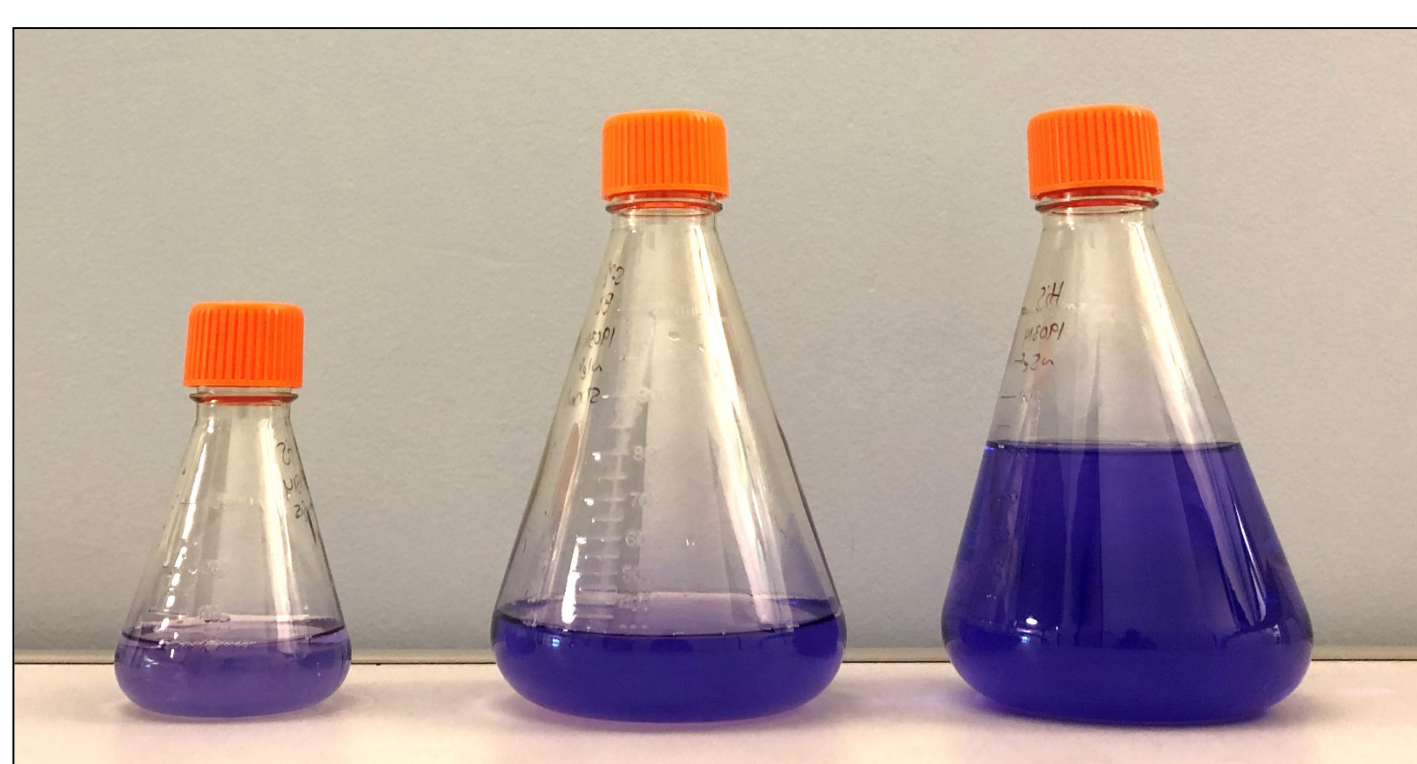
Corning 0.25L Erlenmeyer Flask #431144 0.1L fluid Corning 1L Erlenmeyer Flask #431147 0.3L fluid Corning 1L Erlenmeyer Flask #431147 0.8L fluid
