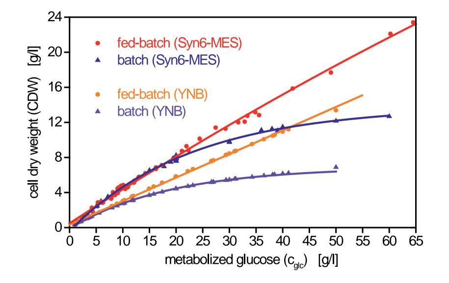
Fig. 2: Cell dry weights of H. polymorpha in batch mode and slow-release fed-batch mode using silicone elastomer discs.
