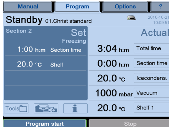
Fig. 65: The freeze-drying process can be started with the aid of the button "Program start".
