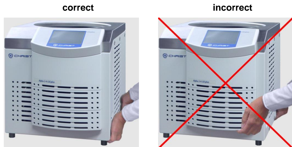
Fig. 9: Lifting the freeze-dryer
