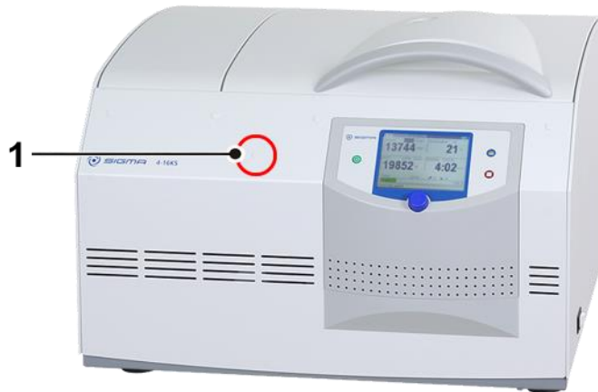
Fig. 31: Position of the opening for the emergency lid release
