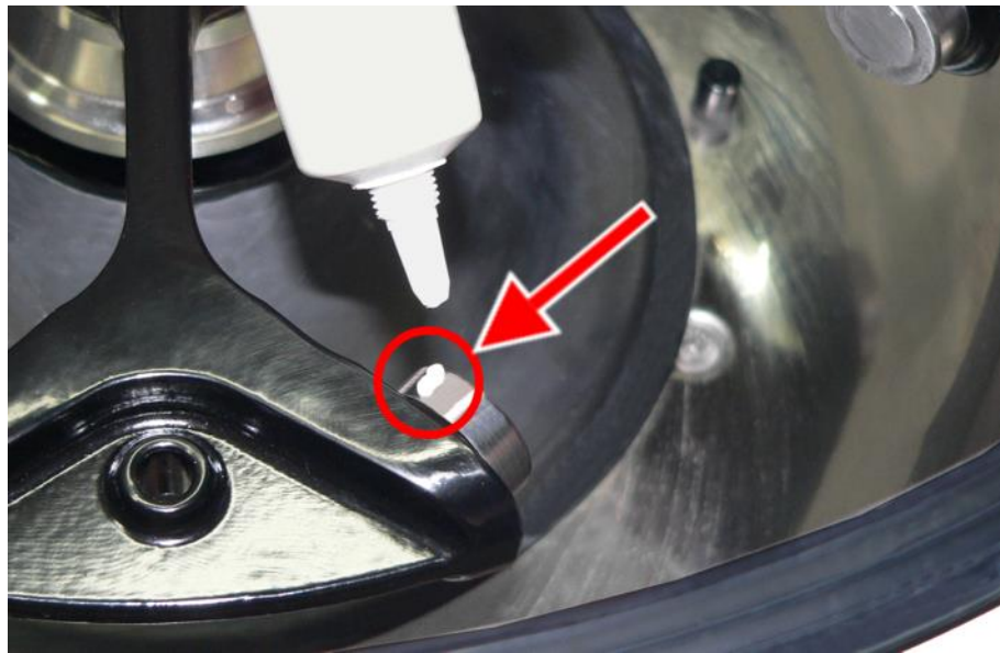
Fig. 34: Sufficient quantity of grease for one bolt
