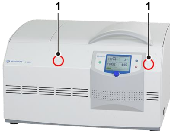
Fig. 32: Position of the opening for the emergency lid release
