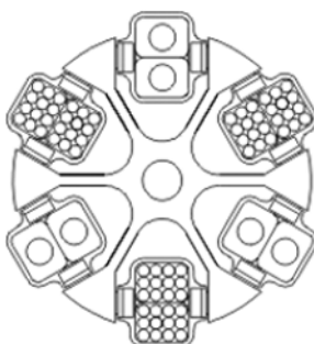
Fig. 8: Permissible and impermissible loading of a swing-out rotor with vessels of various sizes (example illustration)
